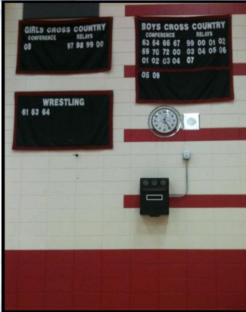
The Noah Instant Box is designed for strength and durability. The cameras are mounted in steel boxes. The camera boxes are mounted inside a larger steel box which also houses the computer and speaker. The door closes with a padlock. The outer cover is designed to handle normal gym activities -- including a direct hit with a baseball.
