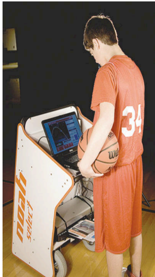
A basketball player checks his stats on the Noah Select System. The system measures the arc of the ball as players shoot to help improve their skills in shooting free throws and three-point baskets.
