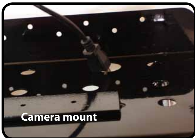
Route the power plug through the large hole. The audio cable can go through the smaller holes.
