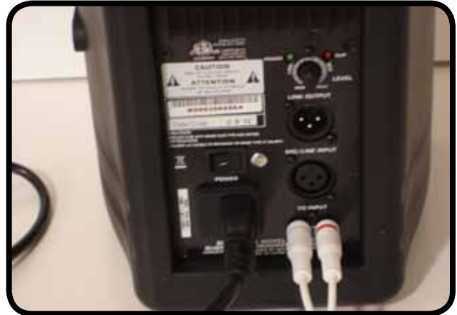
Plug in the power cord and the audio cable (white on white, red on red)
